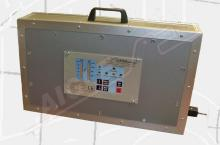
• Electrostatic generator and this is equipped with an "antistalactite" device: in case flock stalactites cause excessive absorption, the generator disconnects itself for a split second, causing the stalactite to fall. This operation is fully automatic and the absorption value after which the unit starts working again can be adjusted.
