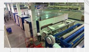
Both the side doors and the top panels are made of galvanized steel containing mineral wool of high density. The oven is constructed to ensure maximum isolation.
