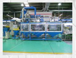
A flock distribution section, consisting of a longitudinal flocking hopper containing a rotating brush. The brush is opposed to a wire mesh frame that can be easily removed for cleaning. Brush rotation speed can be adjusted and a motorized system allows for the adjustment of hopper height, relative to the profile as well.
