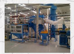
The **Flocking Machine mod. FR1/R** can be used independently or combined, either with one module or more, in order to obtain higher flocking speeds, or with a Flocking Machine mod. FR/ESP for flocking undercut profiles.
