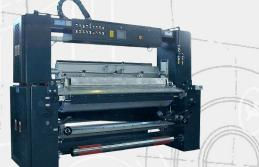
The **Coating Machine mod. BSR/M** is used to coat fabric (with resin and adhesives).
